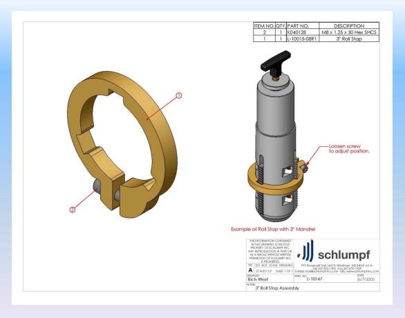
TOGGLE LOCK KEEPS **GRIPPERS IN RETRACTED** POSITION FOR EASIER LOADING AND UNLOADING IN CORE HORIZONTAL POSITION. NOTE! REQUIRES CUSTOMER DISCLAIMER - SCHLUMPF IS NOT RESPONSIBLE FOR DAMAGE OR INJURY IF ROLL IS TURNED TO CORE VERTICAL WHEN TOGGLE IS LOCKED IN RETRACTED POSITON! FOR T-HANDLE & TOGGLE MANDRELS
